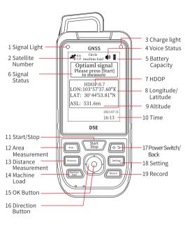
Attention The OK and Direction button in the same position, OK button need press while Direction button need pull.
